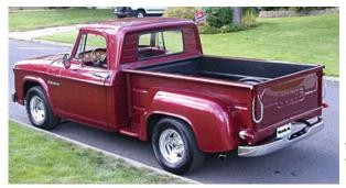
**1961-1965** 1<sup>st</sup> **SERIES SHORT BEDS Dodge completely redesigned their truck line in mid year 1965.** The trucks with the quad headlights are known as 1965 1<sup>st</sup> series and the trucks with the single headlights per side are known as 1965 2<sup>nd</sup> series. Series: 1961 - R, 1962 - S, 1963 - T, 1964-65 1 st - V.
